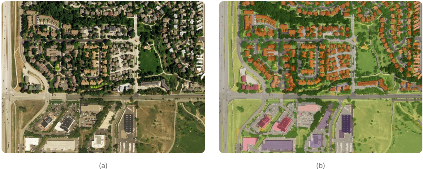
Figure 5. Class precedence where features overlap: (a) the imagery, (b) the final class assigned to each cell.
